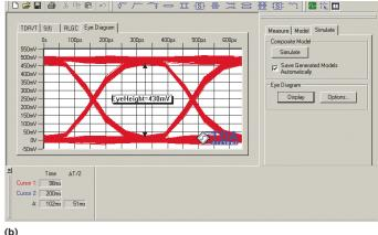
Figure 5 The various trace lengths have eye heights of 500 mV (a) and 430 mV (b). The larger the eye opening, the better the results. Even the worst-case trace has excellent results, well within specifications.
