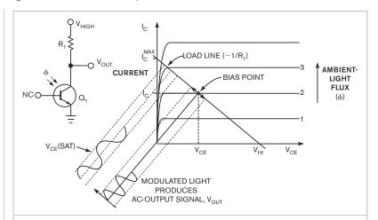
Figure 1 Varying levels of ambient-light flux affect the bias point of a basic phototransistor circuit. Higher levels force the bias point closer to saturation and compress the desired signal,  $V_{\rm OUT}$
