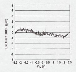
Figure 2. LTC2449 Integral Non-Linearity
