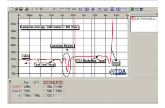
Figure 3 The correlation between simulation and measurement is excellent with equivalent circuit models of a lossy backplane.
