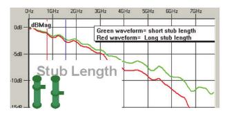
Figure 1 Thicker backplanes use longer via stubs.
