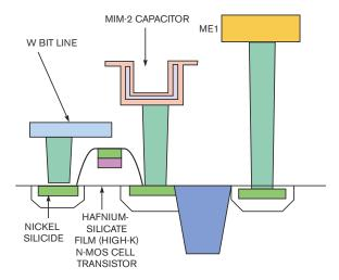
NEC's 55-nm MIM-2 embedded-DRAM cell combines a 0.12-sqmicron area with a 200-MHz system speed.
