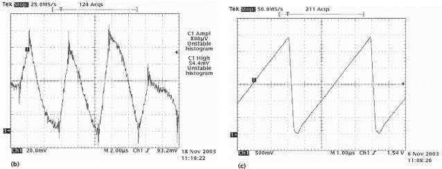
Figure 5 In this inverting buck-boost voltage-mode converter, a common sense-resistor location is in series with the output inductor (a). The sensed-current wavefore (b) is not beautiful but has no nasty current spike. The jagged edges are measuring artifacts. A second oscillogram (c) depicts the sawtooth-oscillator voltage waveform.
