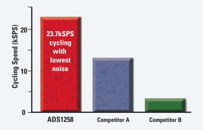
The **ADS1258** 16-channel, 24-bit ADC from Texas Instruments features the lowest latency, fastest channel cycle rate and lowest noise of any competitive devices. With a measurement latency of 42 $\mu$ s, the ADS1258 can measure all of its 16 input channels in less than 675 $\mu$ s with only 12 $\mu$ Vrms of input referred noise, offering unmatched performance for precision, multi-channel data acquisition applications.
