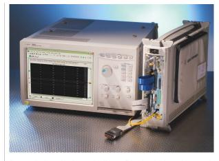
Before the introduction of the E2960B series, logic and protocol analyzers were separate products. The new series combines key features of both into a single product that enables users to understand data from the physical layer to the transaction layer.
