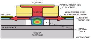
Bonding an indium-phosphide layer over a conventional silicon waveguide, Intel and the University of California-Santa Barbara researchers have demonstrated an electrically pumped laser that requires no precision assembly.
