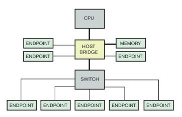
PCI Express replaces the parallel PCI bus with switched serial links containing one or more lanes (courtesy Intel).
