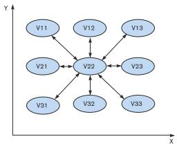
Figure 3 This method compares the voltage of a data point (V22) with its topological neighbors along the X and Y dimensions of the design.
