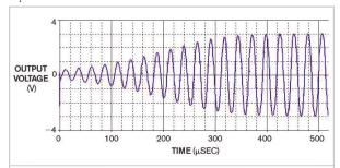
Figure 3 For the component values in Figure 1, the oscillator's output voltage reaches full amplitude in approximately 400 µsec, or 15 cycles after start-up.
