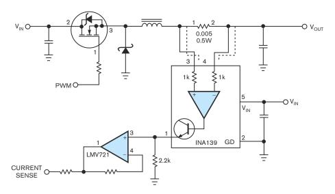
Figure 2 By using a low-valued sense resistor and locating an instrumentation amplifier very near the resistor, you can sense the dc/dc converter's output current with low noise and low power dissipation.
