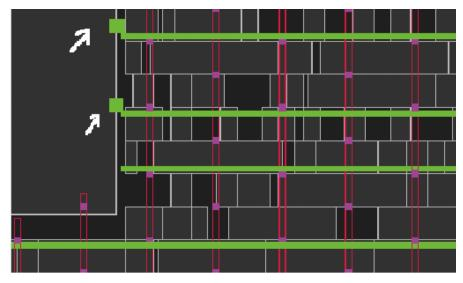
Figure 2 The two pins on the right side of the hard macro barely touch the power rails, resulting in highly resistive connections.
