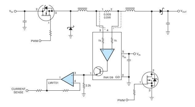
Figure 9 In this noninverting buck-boost converter, the optimal location for the sense resistor and booster-amplifier input is between the two series output inductors.
