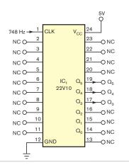
Figure 1 An external 748-Hz clock source drives this PLD-based, three-phase sine-wave generator.
