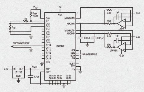
Figure 1. Temperature Sensing Application Example
