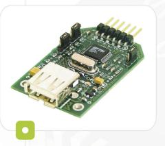
**VDRIVE1** is possibly the easiest solution for adding a USB Flash Drive interface to existing products. Only four signal lines plus 5V/GND are required to be connected.
