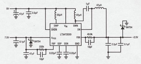
Figure 3. Power Supply for Buffers
