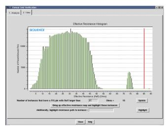
Figure 7 One way to visualize the pins is to create an effective resistance histogram.
