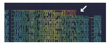
Figure 1 The top three rows of instances connect to power rails supplied by one end only—the power trunk on the left.
