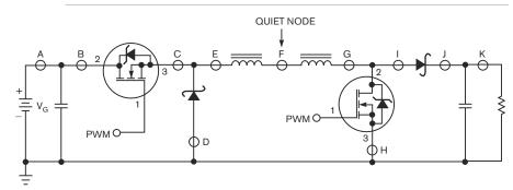
Figure 7 If you can replace the output inductor with two inductors, each having half the value, placing the sense resistor between them yields optimal results.
