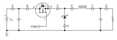
Figure 1 In a buck converter, you can obtain the inductor-current waveform by sensing the power-switch current, which equals the inductor current during the power switch's on-time.
