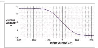
Figure 2 The transfer-characteristic output voltage versus input voltage for the nonlinear amplifier shows a gradual onset of limiting at approximately 100-mV input.
