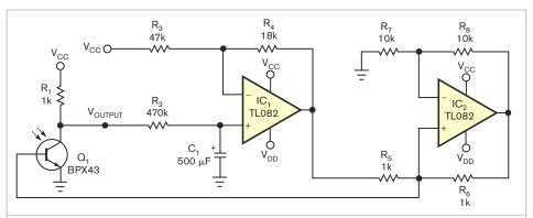
Figure 2 A feedback circuit consisting of a single-pole lowpass active filter and a Howland source diverts current from the phototransistor's base to avoid saturation at excessive background-light levels.
