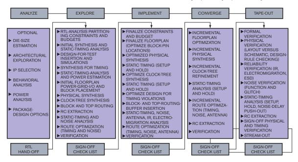
Figure 1 Open Silicon uses a fixed methodology for all its designs.
