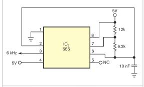
Figure 4 A garden-variety 555 timer IC provides a 6-kHz clock for the switched-capacitor filters.
