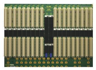
Figure 2 Using a high-grade material, such as the one in this backplane, can provide lower loss-tangent values at high frequencies, translating into cleaner signals.
