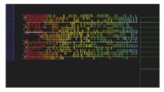
Figure 10 The  $R_{\text{EFF}}$  map and trace-back indicate that only the power trunk on the right side supplies this group, causing it to see high  $R_{\text{EFF}}$ .
