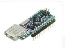
The **VDIP1** module is an MCU to USB Host Controller development module for the VNC1L device and is ideal for rapid prototyping and development of VNC1L designs.
